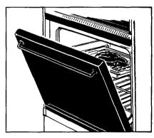
**Step 4:** Leave door open to broil stop position. The door stays open by itself, yet the proper tempera-@ is maintained in the oven.
